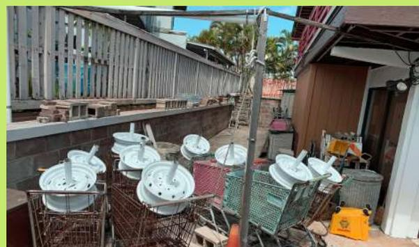
Old car rims were cleaned of rust, primed and painted - - to be made into stanchions for New Years day
