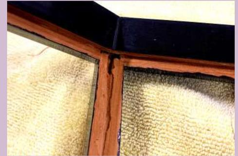
The lamp frames were then inspected for further damages. Termite damage was found in several of the lamp shades, creating channels into the wooden frame.
