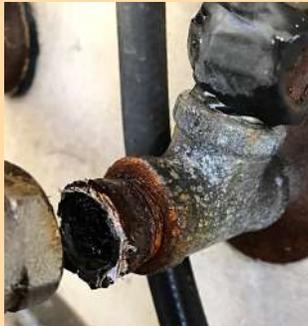
Corrosion caused one of the exterior faucets to break off the fixture.
